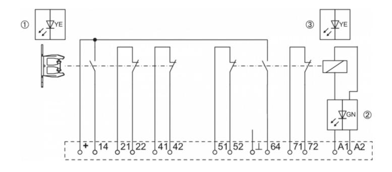
The 24 V are led internally to contacts 13 and 63. The corresponding signals of the LED display can also be tapped at terminals 14 or 64.
