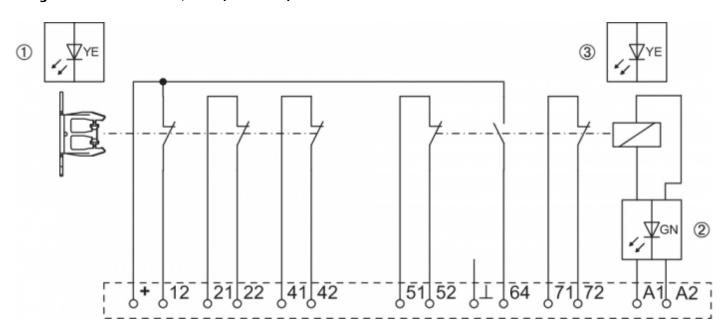
The 24 V are led internally to contacts 11 and 63. The corresponding signals of the LED display can also be tapped at terminals 12 or 64.
