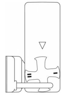
The diagrams show a closed guard system with a set latching force of 50 N (see also chapter "adjustment of latching force").
