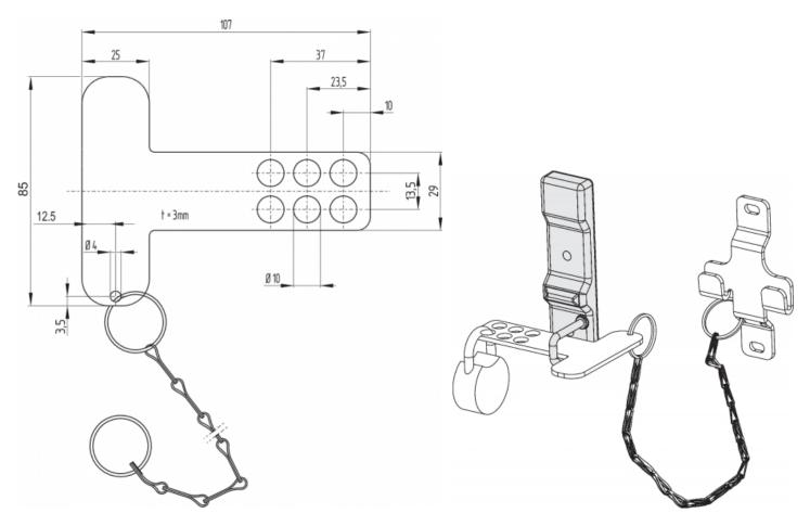
**Bowden cable release ACC-AZM300-BOW-.-.M-.M (available as accessory)** Observe the additional notes in the operating instructions of the Bowden cable release.
