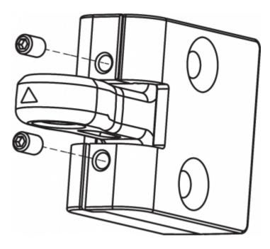
The hexagon socket screws must not be completely unscrewed.
