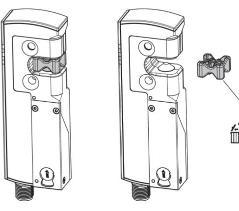
For attachment of the solenoid interlock and the actuator, two mounting holes for M5 screws are provided.
