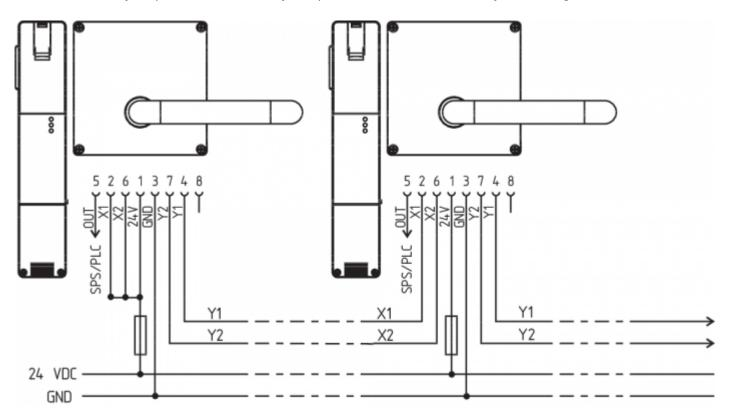
Y1 and Y2 = Safety outputs  $\rightarrow$  Safety monitoring module
