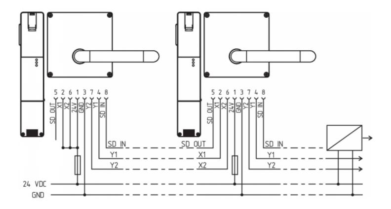
Y1 and Y2 = Safety outputs  $\rightarrow$  Safety monitoring module SD-IN  $\rightarrow$  Gateway  $\rightarrow$  Field bus
