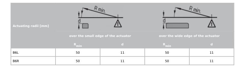
The axis of the hinge must be d mm above and in a parallel plane to the top surface of the safety switch. The basis setting provides a minimum radius of  $R_{\min}$ .
