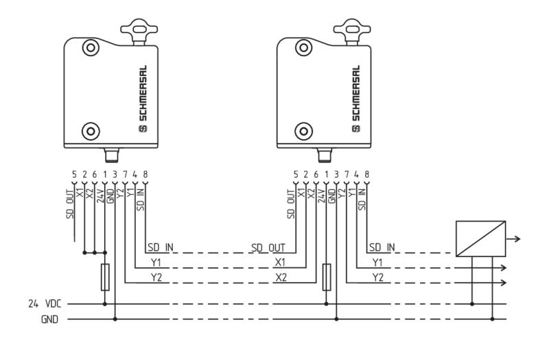
Y1 and Y2 = Safety outputs  $\rightarrow$  Safety monitoring module SD-IN  $\rightarrow$  Gateway  $\rightarrow$  Field bus
