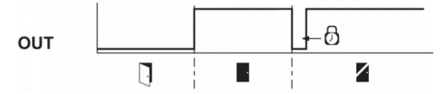
Door could not be locked or fault
