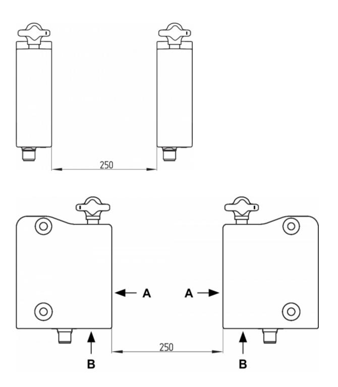
The minimum distance from metallic securing surfaces to the face side "A" and underside "B" of the device is 5 mm.
