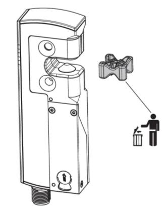
For attachment of the solenoid interlock and the actuator, two mounting holes for M5 screws are provided.
