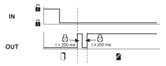
Disrupted process, door could not be locked or error
