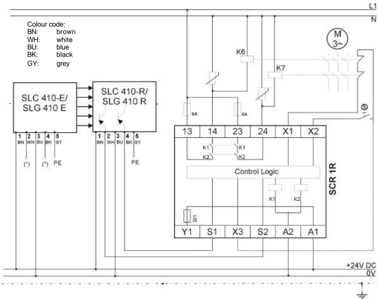
\* Refer to table 2, page 10 for the correct connection of pins 2 and 4
