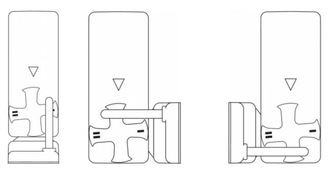
The diagrams show a closed guard system with a set latching force of 50 N (see also chapter "adjustment of latching force").
