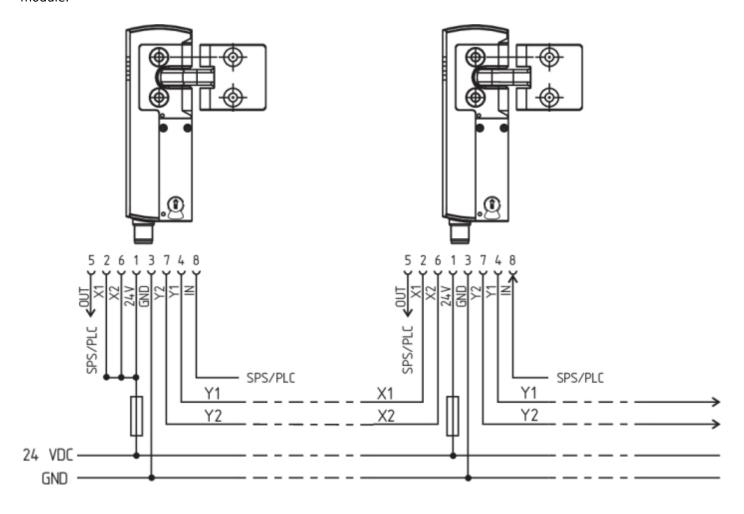
Y1 and Y2 = Safety outputs → Safety monitoring module
