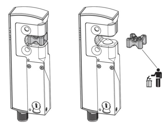
For attachment of the solenoid interlock and the actuator, two mounting holes for M5 screws are provided.
