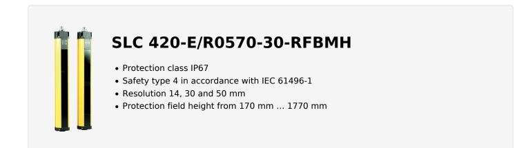
Schmersal India Pvt. Ltd., Plot No - G-7/1, Ranjangaon MIDC, Tal. - Shirur, Dist.- Pune 412 220 The details and data referred to have been carefully checked. Images may diverge from original. Further technical data can be found in the manual. Technical amendments and errors possible. Generated on: 29/11/2024, 7:31 am
