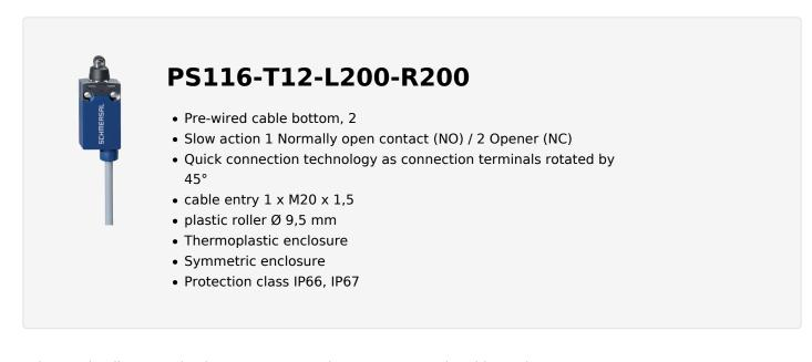
Schmersal India Pvt. Ltd., Plot No - G-7/1, Ranjangaon MIDC, Tal. - Shirur, Dist.- Pune 412 220 The details and data referred to have been carefully checked. Images may diverge from original. Further technical data can be found in the manual. Technical amendments and errors possible. Generated on: 03/12/2024, 8:04 pm
