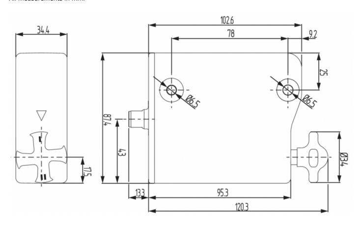
**AZM300...-T/-T8 and -N**Device with emergency exit or emergency release
