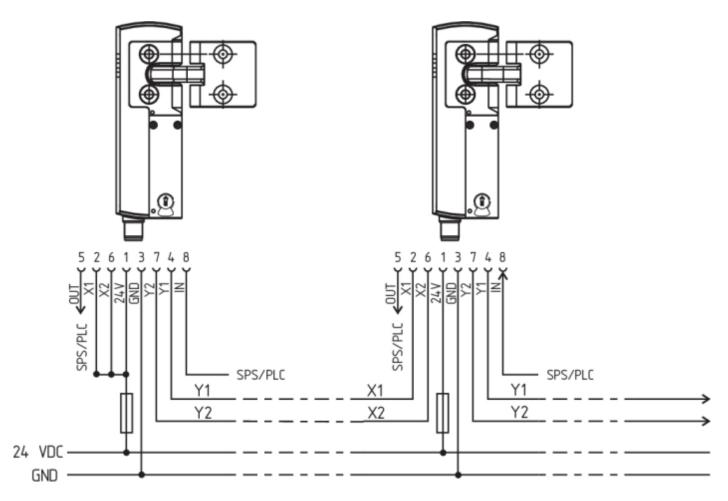
Y1 and Y2 = Safety outputs  $\rightarrow$  Safety monitoring module
