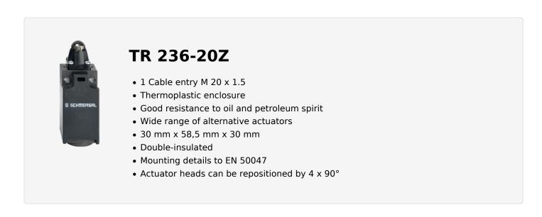
K.A. Schmersal GmbH & Co. KG, Möddinghofe 30, 42279 Wuppertal The details and data referred to have been carefully checked. Images may diverge from original. Further technical data can be found in the manual. Technical amendments and errors possible. Generated on: 06/05/2025, 18:30
