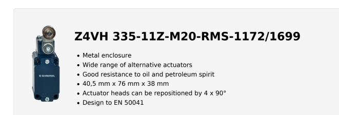
K.A. Schmersal GmbH & Co. KG, Möddinghofe 30, 42279 WuppertalThe details and data referred to have been carefully checked. Images may diverge from original. Further technical data can be found in the manual. Technical amendments and errors possible.Generated on: 07/06/2025, 15:15
