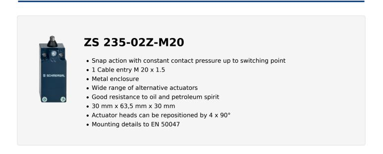
K.A. Schmersal GmbH & Co. KG, Möddinghofe 30, 42279 Wuppertal The details and data referred to have been carefully checked. Images may diverge from original. Further technical data can be found in the manual. Technical amendments and errors possible. Generated on: 01/07/2025, 04:07
