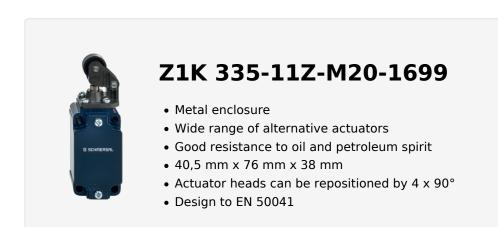
K.A. Schmersal GmbH & Co. KG, Möddinghofe 30, 42279 WuppertalThe details and data referred to have been carefully checked. Images may diverge from original. Further technical data can be found in the manual. Technical amendments and errors possible.Generated on: 20/07/2025, 21:00
