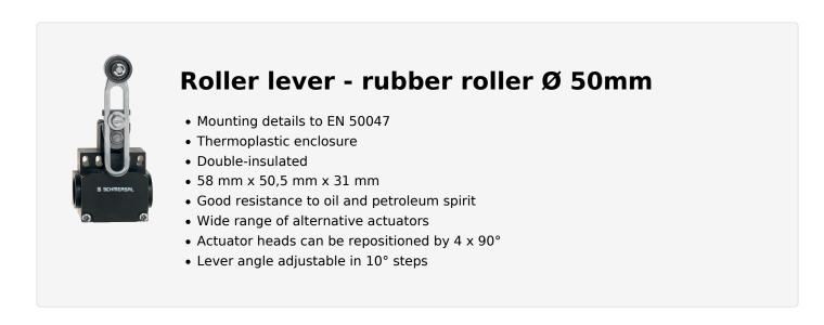
K.A. Schmersal GmbH & Co. KG, Möddinghofe 30, 42279 Wuppertal The details and data referred to have been carefully checked. Images may diverge from original. Further technical data can be found in the manual. Technical amendments and errors possible. Generated on: 10/04/2025, 21:46
