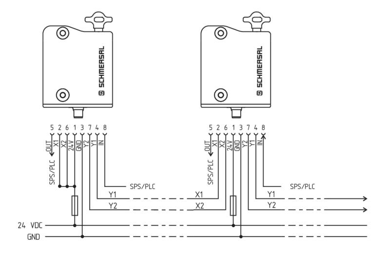
Y1 and Y2 = Safety outputs → Safety monitoring module
