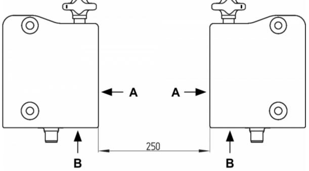
The minimum distance from metallic securing surfaces to the face side "A" and underside "B" of the device is 5 mm.
