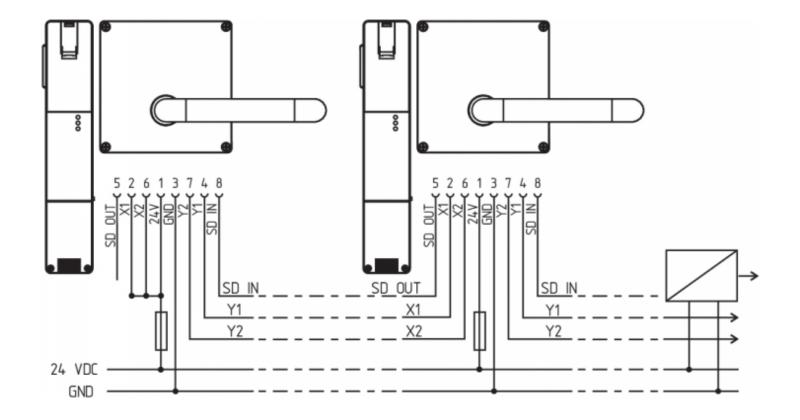
Y1 and Y2 = Safety outputs → Safety monitoring module SD-IN → Gateway → Field bus
