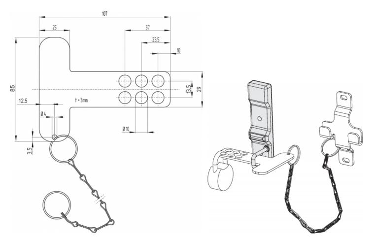
Bowden cable release ACC-AZM300-BOW-.-.M-.M (available as accessory)
