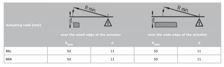
The axis of the hinge must be d mm above and in a parallel plane to the top surface of the safety switch. The basis setting provides a minimum radius of  $R_{\min}$ .
