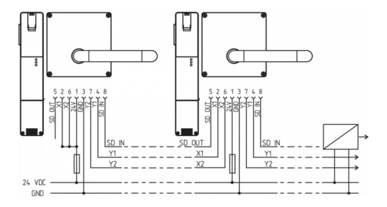
Y1 and Y2 = Safety outputs  $\rightarrow$  Safety monitoring module SD-IN  $\rightarrow$  Gateway  $\rightarrow$  Field bus
