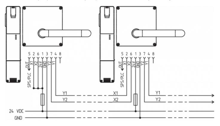
Y1 and Y2 = Safety outputs → Safety monitoring module
