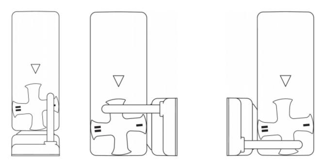
The diagrams show a closed guard system with a set latching force of 50 N (see also chapter "adjustment of latching force").
