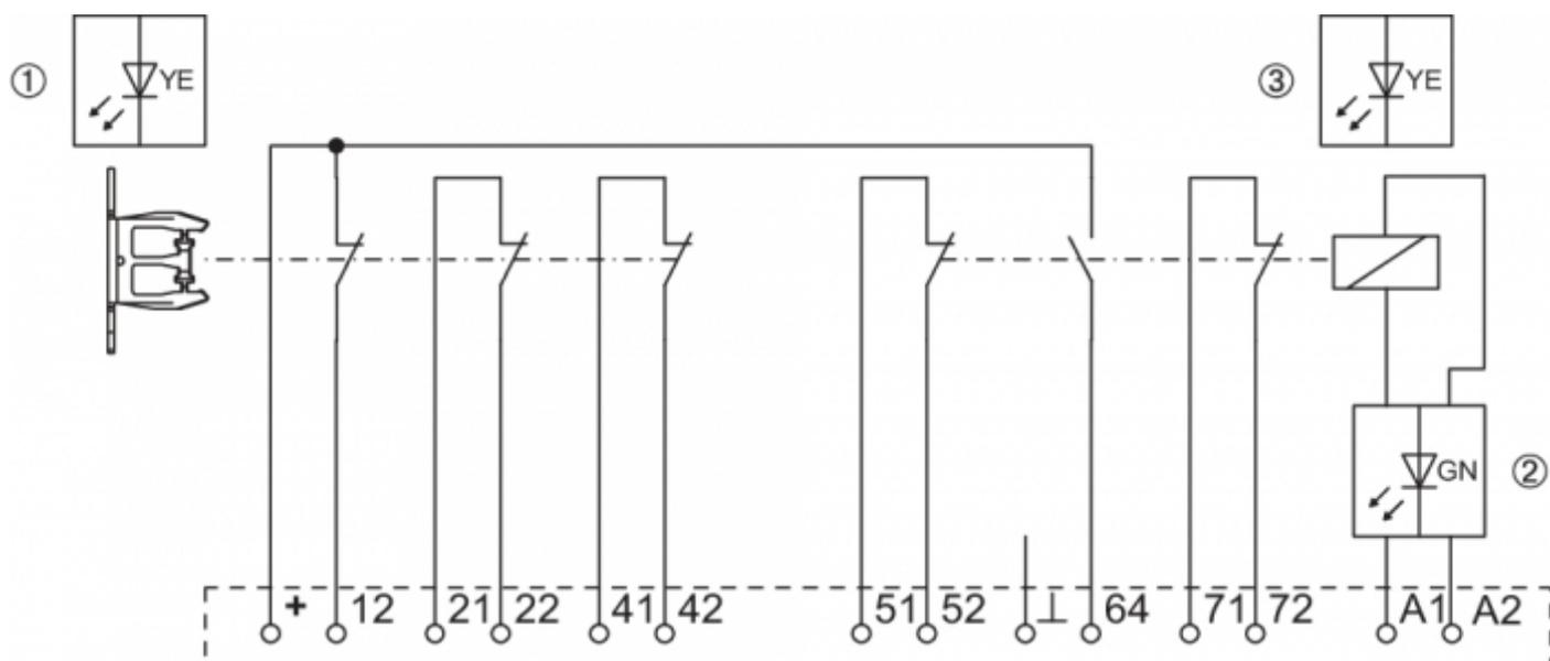
The 24 V are led internally to contacts 11 and 63. The corresponding signals of the LED display can also be tapped at terminals 12 or 64.
