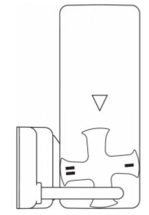
The diagrams show a closed guard system with a set latching force of 50 N (see also chapter "adjustment of latching force").
