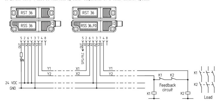
Wiring example 4: Series-wiring with RSS 36...F1-Q as master with EDM
