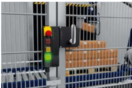
Fig. 2: The components of a practical safety solution. A view of the process, operating elements close to the door handle, information about the operating state of the safety switchgear device.
