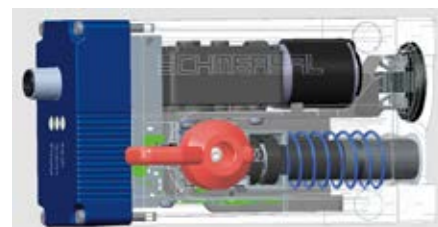
Fig. 2: The AZM400 safety interlock comprises the interlock unit with sensor system, a motor-driven locking bolt and an actuator. This contains an encoded RFID tag and a catch opening into which the locking bolt is inserted.
