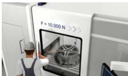
Fig. 1: The AZM400 safety interlock has a holding force of 10 000 N
