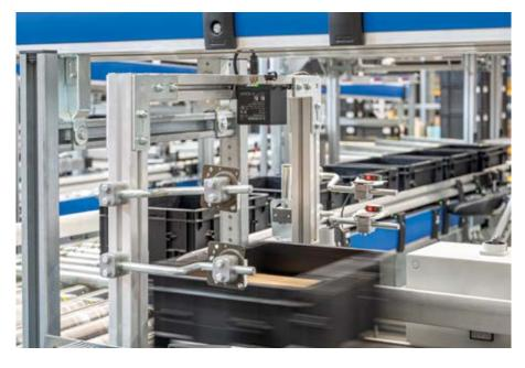
The AM-T100 is equipped with a Sony DepthSense sensor and uses Time-of-Flight (ToF) technology – the runtime measurement of emitted light pulses within the infrared range (850 Nm), which are reflected by the objects being detected. This enables high-speed creation of a 3D image of the scene with millimetre accuracy that is available as a point cloud.
