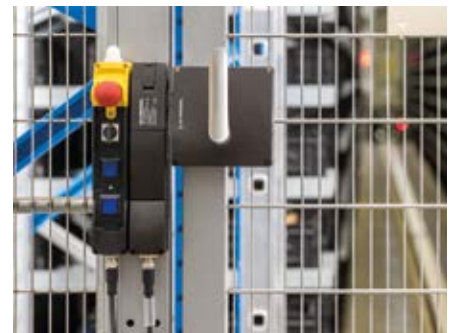
Fig. 1: The combination of door handle, safety switching device and operating/display elements has already proved its worth.
