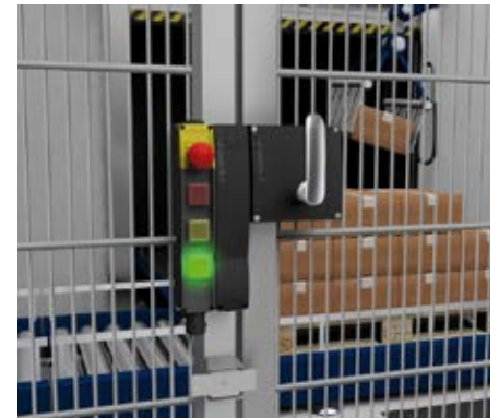
The data collected from safety switchgear by the safety controller can be forwarded to higher-level control room via OPC UA and utilised for predictive maintenance.
