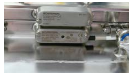
Fig. 2: Depending on the application – here on a system for pharmaceutical production – non-concealed, coded safety sensors are also used
