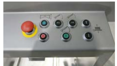
Fig. 1: Developed for machines in the food industry: the hygiene-compliant operating and control devices in the N programme
