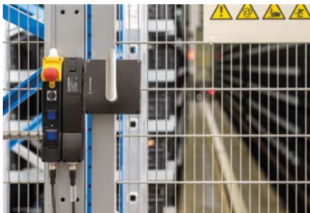
Fig. 1: Solenoid interlocks such as the AZM201 from Schmersal are used to monitor the position of safety gates, e.g. at robot workstations. The AS-i Safety at Work safety bus can be used to integrate solenoid interlocks and operator interfaces into a safety circuit.
