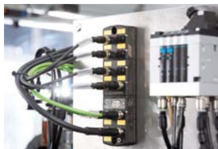
Fig. 3: Range expansion: a new Safety Fieldbox also communicates via the EtherNet/IP with CIP Safety and EtherCAT with FSoE bus systems.
