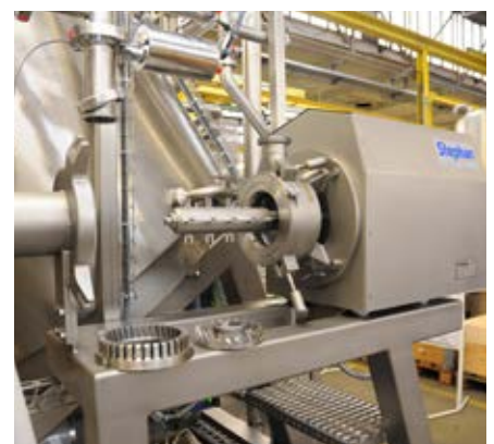
Fig. 3: The Microcut is installed in a robust stainless steel casing and has various cutting tools.
