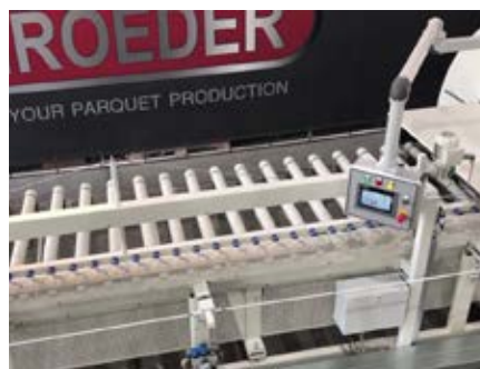
There are some 15 to 20 emergency stop buttons on the system, so it is important that the safety controller can forward diagnostic data to the operating controller.
