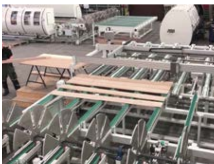
Schroeder's machine line for profiling polished multi-layer parquet uses the modular PROTECT PSC1 safety controller from Schmersal.
