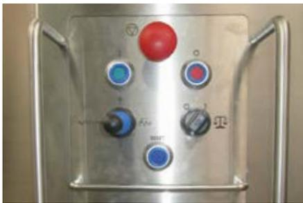
The NK cross switch, at the bottom left of the control panel, can be moved to up four positions: top, bottom, right, left.
