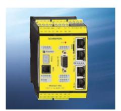
Safety in system: The signals from the SLB range can be evaluated by the new modular Protect PSC 1 safety controller, for example.
