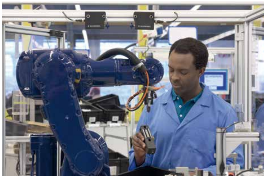
The "beyondSpai" project is addressing the improved protection of the collaboration between man and robots. Optical sensors and special image processing algorithms are to detect human skin and to identify human silhouettes
