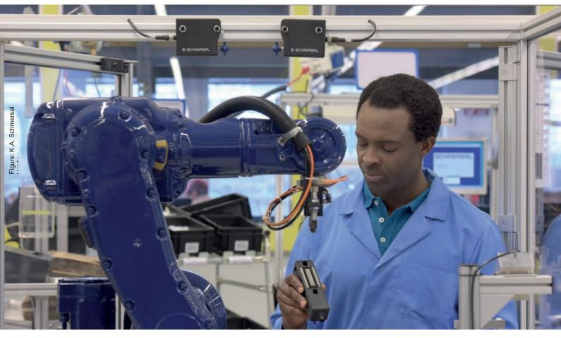
State of technology in Industry 4.0 production: Cooperation between humans and robots without safety fences
