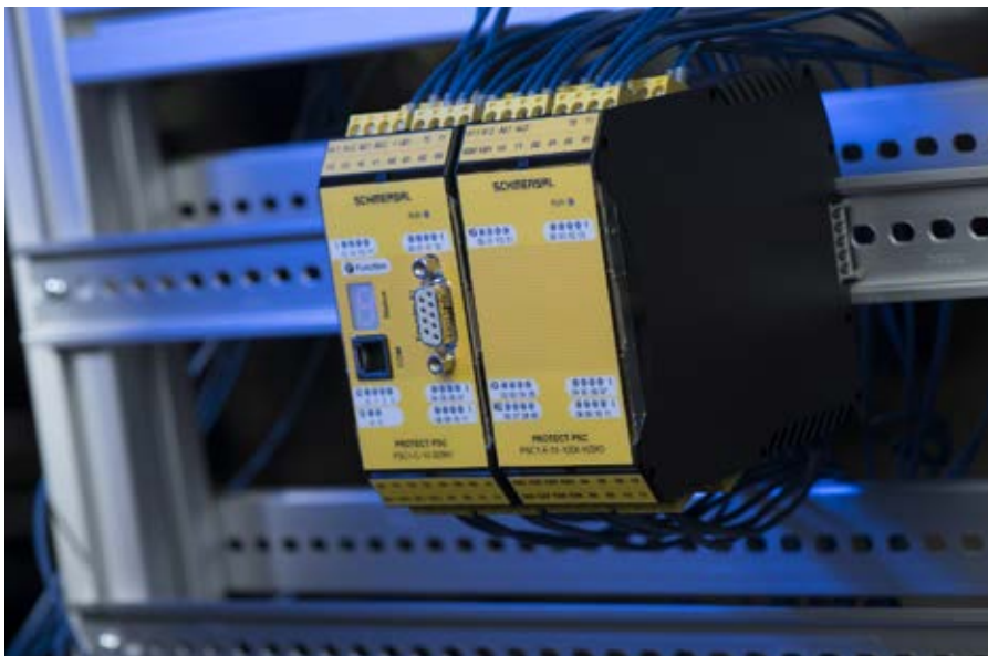
Fig. 2: The Protect PSC1 safety controller enables the realisation of 'safety separated' solutions. It also enables integration into higher-level infrastructure.
