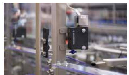
Fig. 2: Siléane uses AZM300 series solenoid interlocks to safeguard hazardous areas
