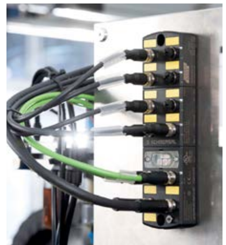
Fig. 2: Simple plug & play solution: the new Safety Fieldbox from Schmersal
